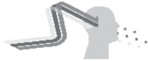
FIGURE 1. In conventional radiography the exit dose may be only 1% of the entrance dose.
